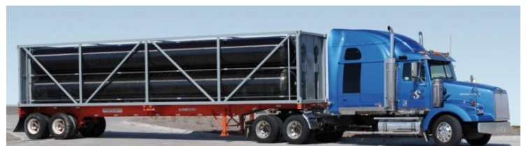
Titan tube trailer for CNG storage and distribution
