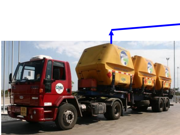
CNG storage and distribution system supplied by Galileo
